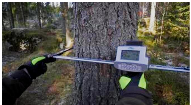
使用 Masser 测径仪进行样地信息采集和树木测量 Site information and tree measurements was made with Masser measuring scissors
